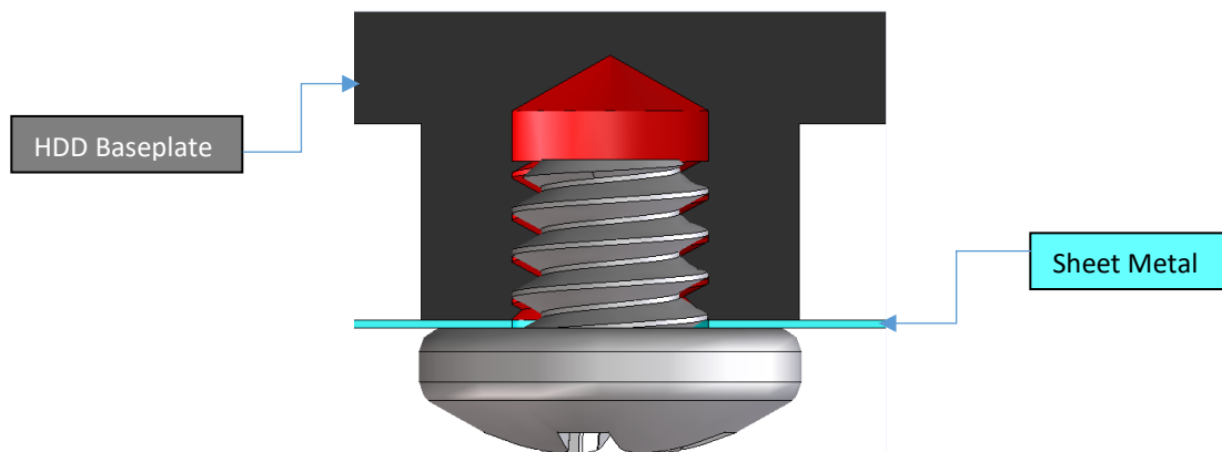
Figure 6. Bottom mount hole, 6-32UNC X 1/8" (3.8 threads engagement)
